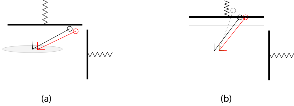
Figure 5.5: This figure depicts the second stage of the example equality constrained problem. After moving out of contact with the environment (shown in (a)), the arm moves into contact a second time (shown in (b)), which shrinks the uncertainty.
