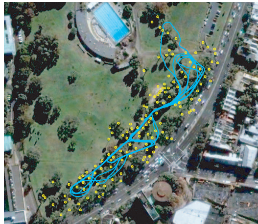
Fig. 8. An experimental result of bearing only SLAM using the Victoria Park dataset. A solid line depicts the robot trajectory and yellow dots depict landmarks.
